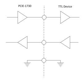
Figure 3.2 TTL-Level DI/O Connection
