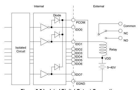
Figure 3.5 Isolated Digital Output Connection
