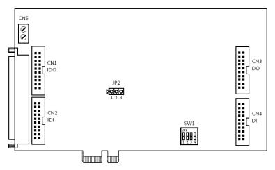
Figure 3.1 Card Connectors, Jumpers, and Switches
